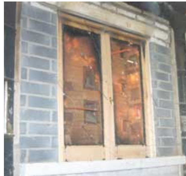
FIRESTILE doors under test at Warrington Fire Research Centre
